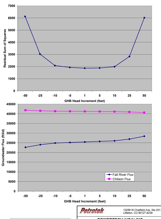
Groundwater Flux Measured at Location Indicated on Figure 5-9
