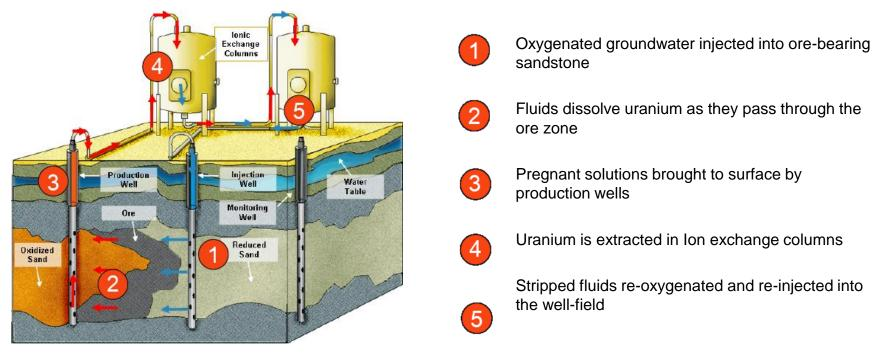
Recycling fluids through the well-field is an efficient, non-consumptive use of groundwater. Up to 90% of in-place uranium is recovered
