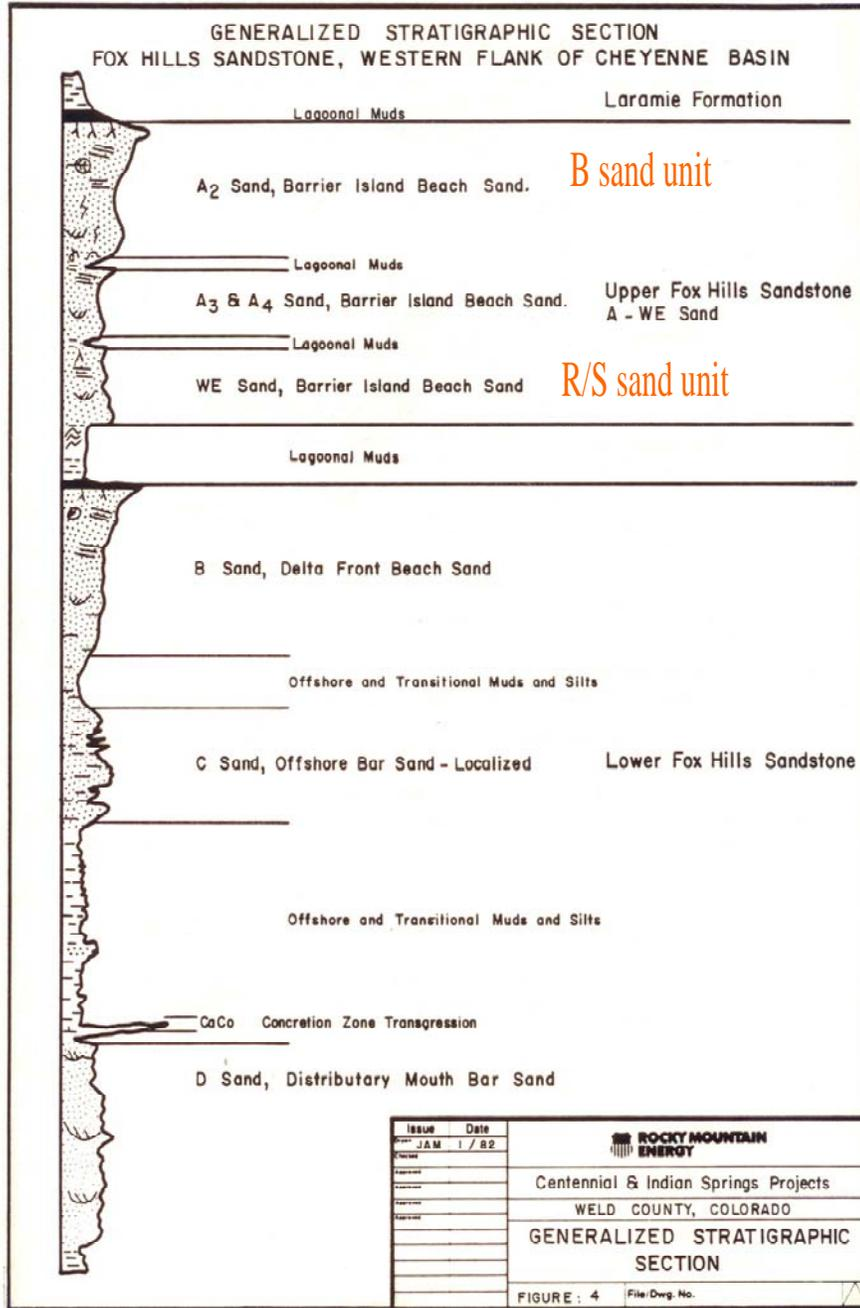
Figure 8 Generalized Stratigraphic Section of Centennial Project host rocks
